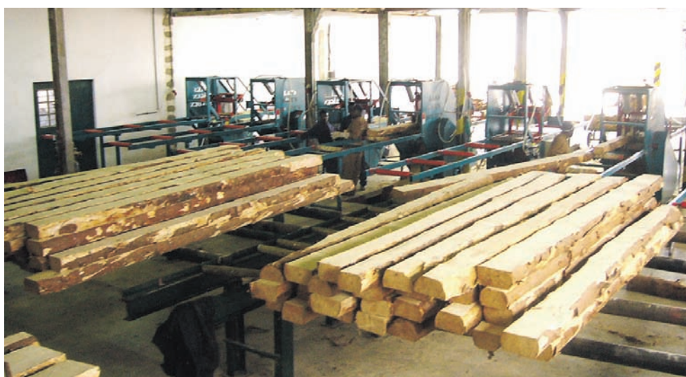
• The frame sawmill Logosol-Laks is a simple and stable construction with high capacity and high accuracy, and it leaves a very clean cut. The frame saws were placed side by side with a roller-track system.
