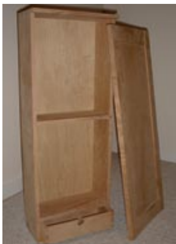
Cherry Shaker Wall Cabinet. Frame and panel door; dovetailed drawer; sliding dovetail shelves.
