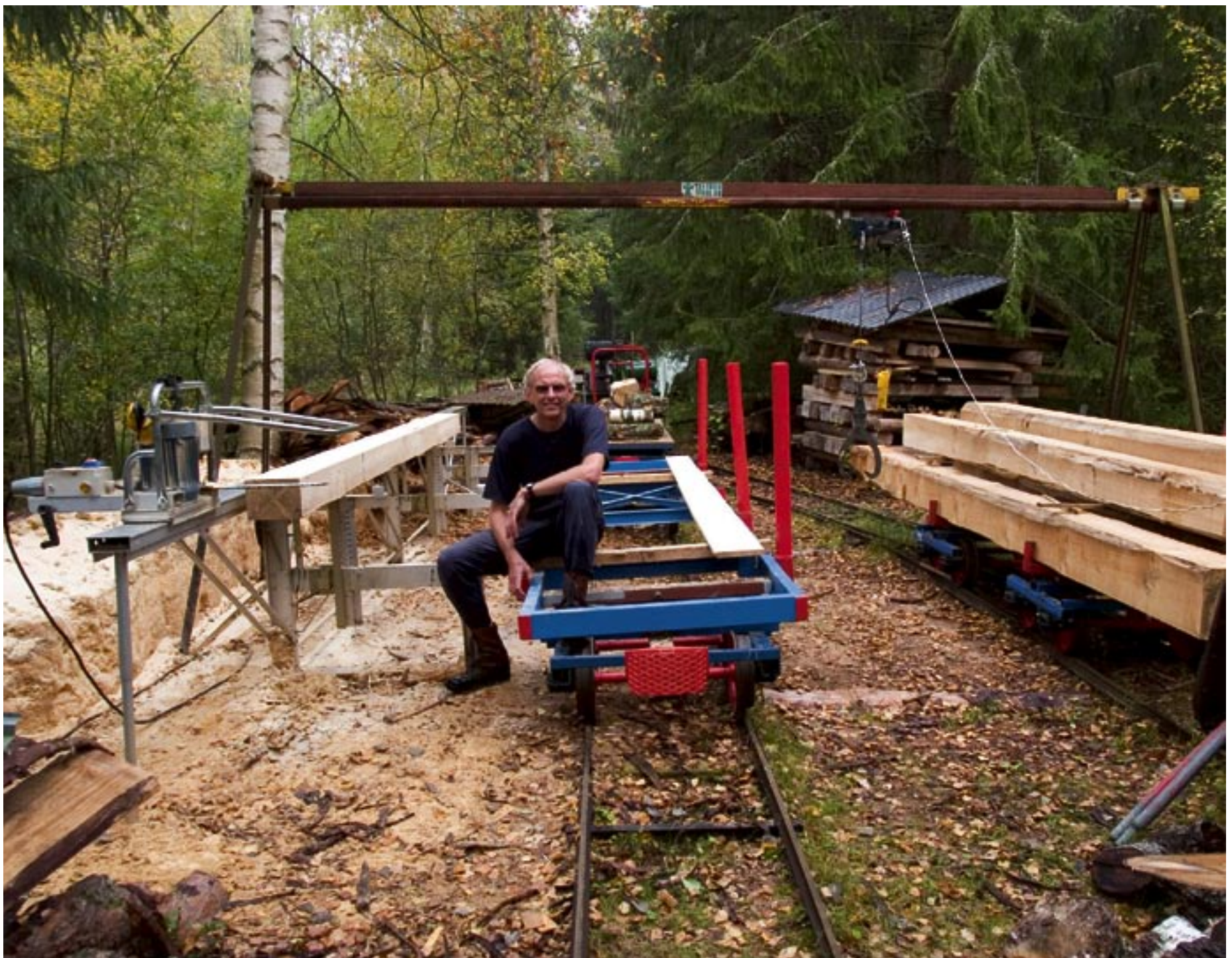
Bo Malmberg works as a production technology manager at Electrolux in Motala, so it is not surprising that the logistics around the sawmill are well thought out. The logs arrive on the track to the right. Then, they are lifted onto the Logosol Sawmill with the help of the electric gantry crane. Finally, the boards and planks are placed on the wagon to the left and transported to be seasoned.
