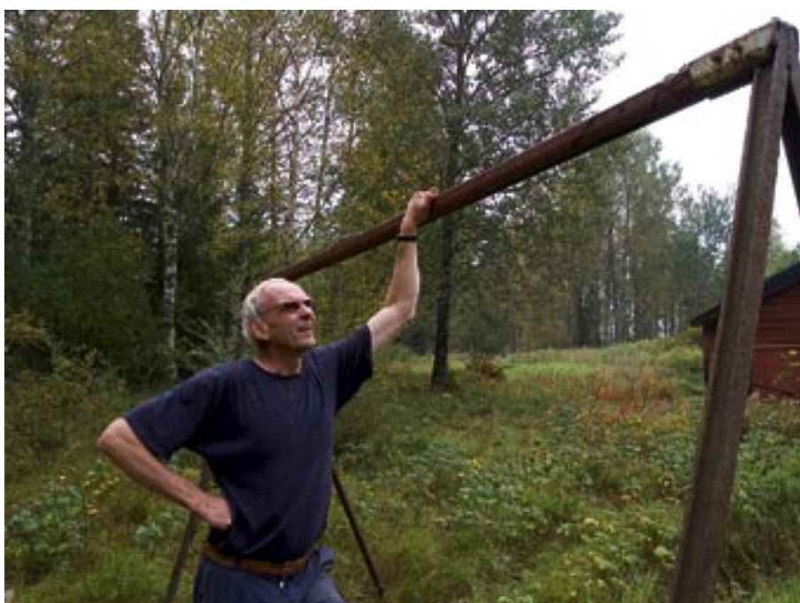
Bo Malmberg recommends using a gantry crane for lifting logs. He himself has two, and this one is portable.
