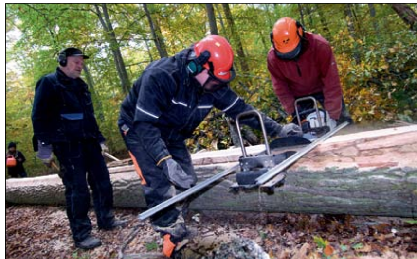
The Logosol Big Mill LSG can handle long logs of really large diameters.
