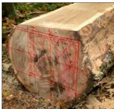
The soon-to-be keel marked out on the log end.
