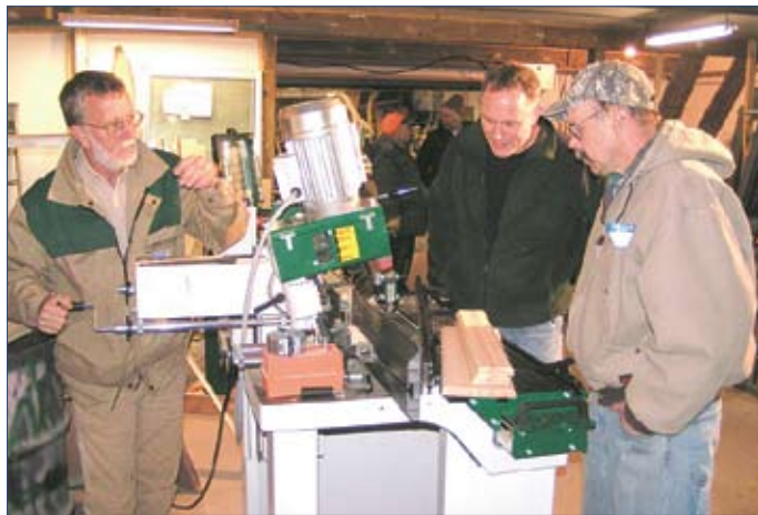
Charlie Griffin demonstrates the tilting head on the Logosol MF30 spindle shaper.
