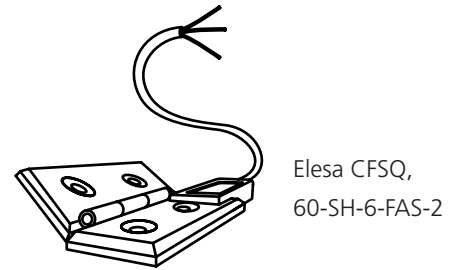
Interlock safety switch
