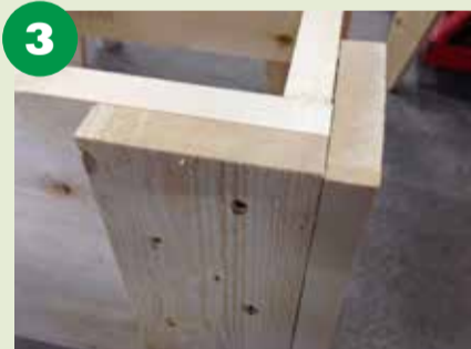
• As cover boards, we used the same planed boards as we used for decoration.
