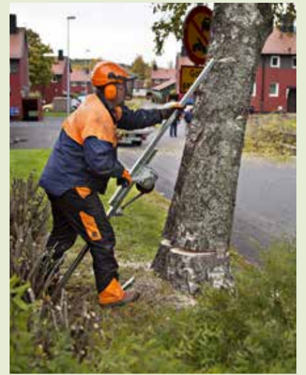
• The Tree Pusher from LOGOSOL ensures that the tree falls in the intended direction. See video on logosol.co.uk .
