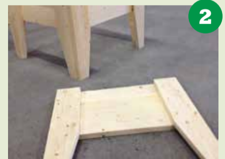
• The legs were made bevelled before we nailed the pieces together. (Using screws works just as well.)
