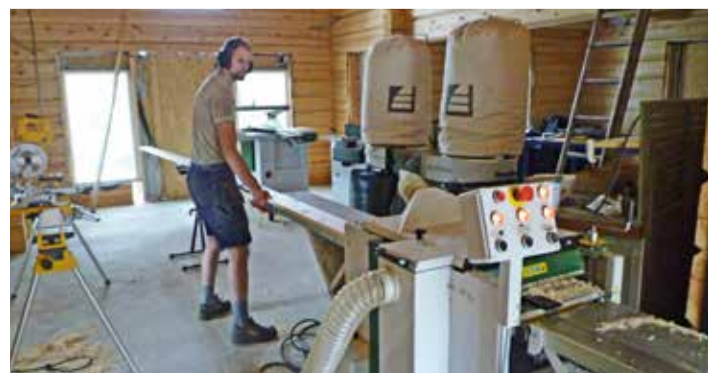
• Time for joinery! The joinery machines have been taken indoors for production of windows and interior joinery. Christian Sämberg is working by the planer/moulder.
