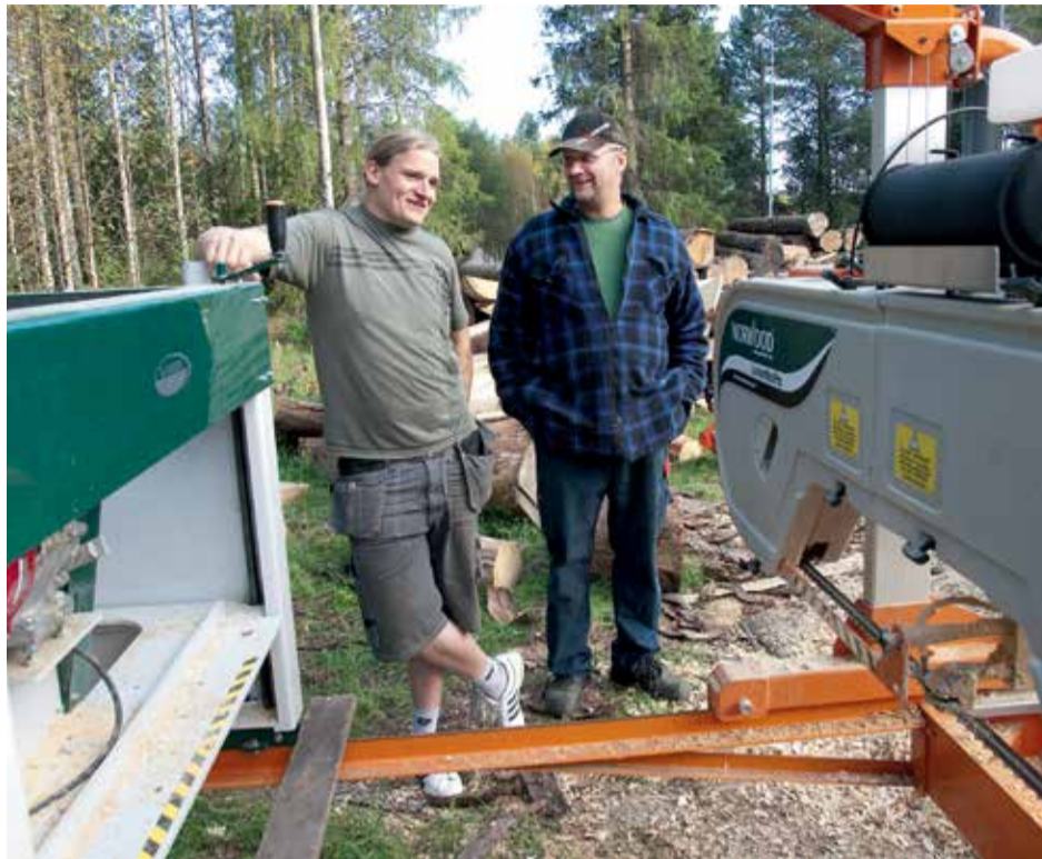
• The combination band sawmill and log moulder from Logosol is perfect for producing log houses of over-sized logs, David Nilsson and Tomas Broström think.
