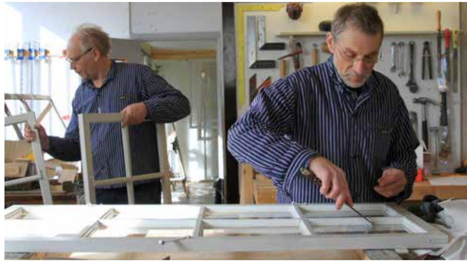
At OscarsHus windows are manufactured with inspiration from skilled craftsmen from of the past. With pine heartwood, linseed oil paint and wooden dowels the result becomes both beautiful and durable.
