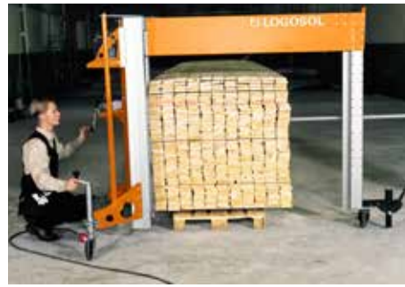
Just in time for the 10-year anniversary, a mobile stack cutter for precision cutting of timber packs.
