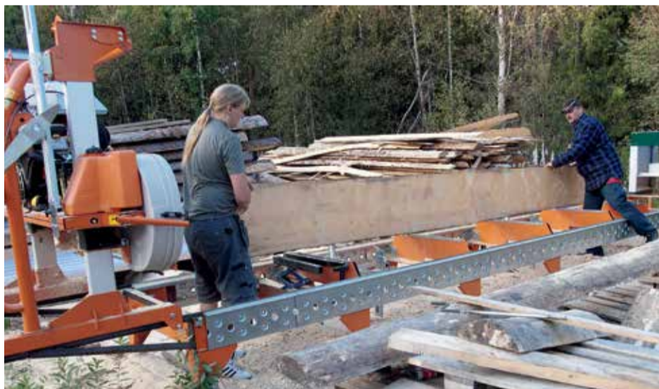
• The sawmill can without problem handle logs that are 70 centimetres in diameter.
