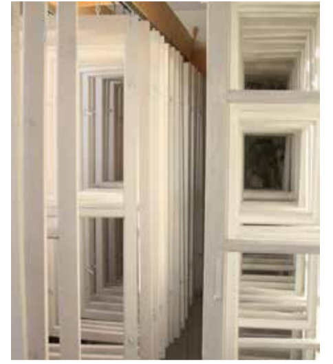
At OscarsHus windows are manufactured with inspiration from skilled craftsmen from of the past. With pine heartwood, linseed oil paint and wooden dowels the result becomes both beautiful and durable.
