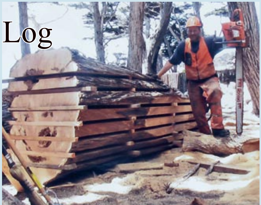
Rob next to California Cyprus log stacked to dry in original log shape Japanese style, log cut using the M-7 in inversion fashion
