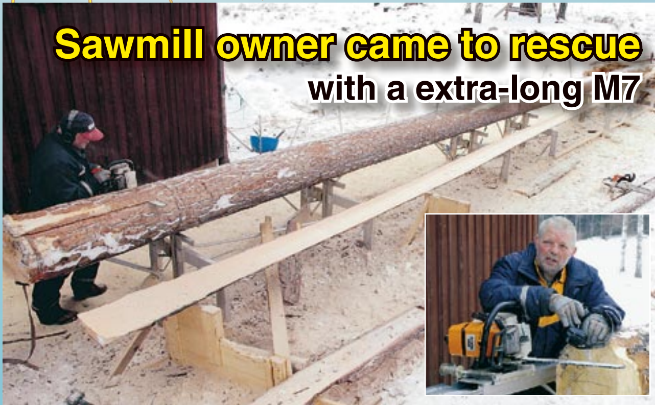
Poul Nielsen (inset) with an extraordinary sawmill! Three and a half M7s were the only way that the 17-metre long, ruler straight beams could be cut out for use in rebuilding the church tower.
